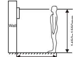
[Suggestion]: The camera should be 1450~1550mm above the ground. The camera at this height can capture human face perfectly.
